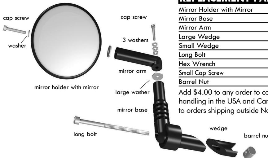
**position the mirror base so that the top tilts further down and out of the way of the bar end.** Use the hex wrench that is included to tighten the bolt until the mirror base is secure in the end of the handlebar.
